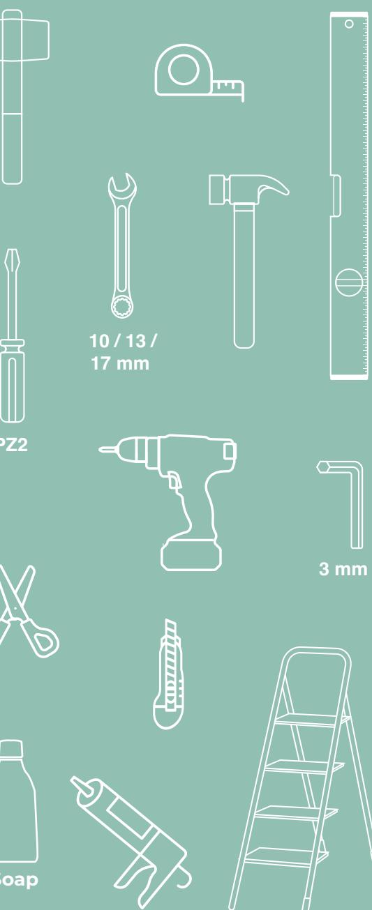
**UK:** Necessary tools – rubber mallet, measuring tape, spirit level, screwdriver PZ2, wrenches 10/13/17 mm, cordless drill, 3 mm hex key, utility knife, \*soap for rubber when oil is not enough, silicone gun and silicone, ladder.
